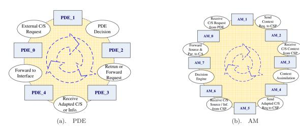
Figure 3. PDE and AM's Working Cycle
